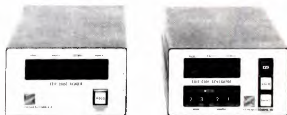
Fig. 2. Compact Edit Code Generator & Reader make possible tape search, interlock of machines and videotape electronic editing. Photo courtesy Stephens Electronics
