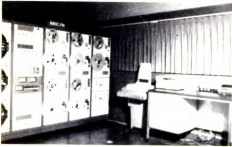
Sono-Mag DP-1 at WROC, Rochester, has five Scully tape decks (right hand bays), three Carousels (left end), with control equipment in center including full random access, and storage of 2048 events.
